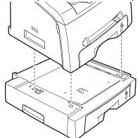
5 Plug the interface cable of the tray into the Tray 2 cable connector on the back of the machine.
